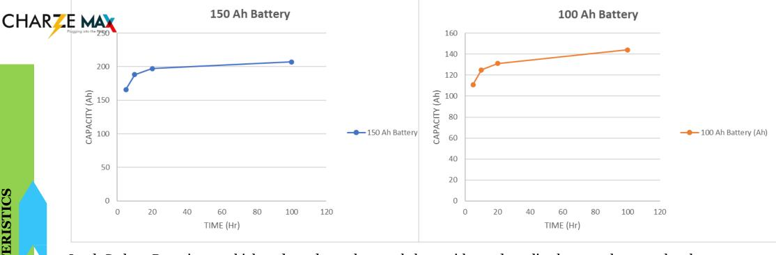
Lead Carbon Batteries are high-end products that work best with good quality battery chargers that have a compatible charge profile (or ability to adjust custom charge settings). Below settings for automated battery chargers are recommended to fully utilize the benefits of Lead Carbon Batteries.
